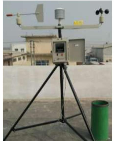
Data logger has facility to transfer data either through SD card or optional RS 232/485 to USB modbus. Memory of the logger is enough to record more than 4 months meteorological data with log frequency of 1hr for all sensors. A windrose preparation software is provided with each WM 721 using which coloured circular wind rose diagram can be drawn for required period. All data from logger is transferred in Excel sheet. Software is with any operating system equipped with MS Excel.
